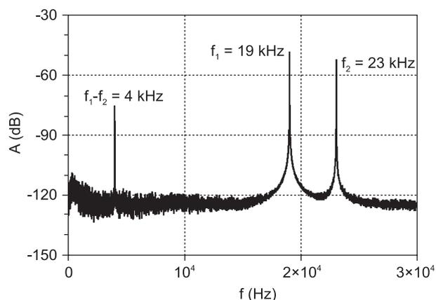
Figure 10. Response frequency spectrum obtained from a damaged ceiling slab, two exciting signals.
