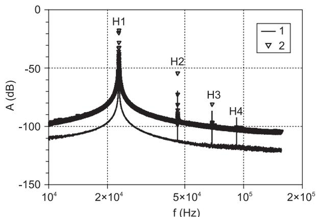
Figure 7. Response frequency spectra of an undamaged ceiling slab, single exciting signal.
