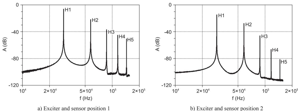
Figure 4. Response frequency spectra of an undamaged specimen B1.
