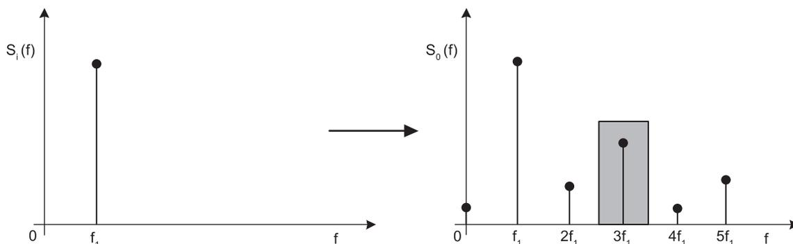
Figure 1. Growth higher harmonic components in frequency spectra at transit pure harmonic signal through nonlinear environment with illustration of dominant third harmonic component selection by the frequency band-pass filter.
