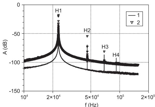
Figure 7. Response frequency spectra of an undamaged ceiling slab, single exciting signal.
