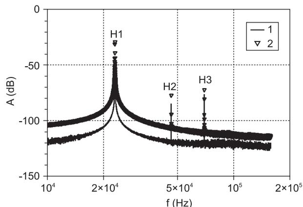
Figure 9. Response frequency spectra of a damaged ceiling slab, single exciting signal.
