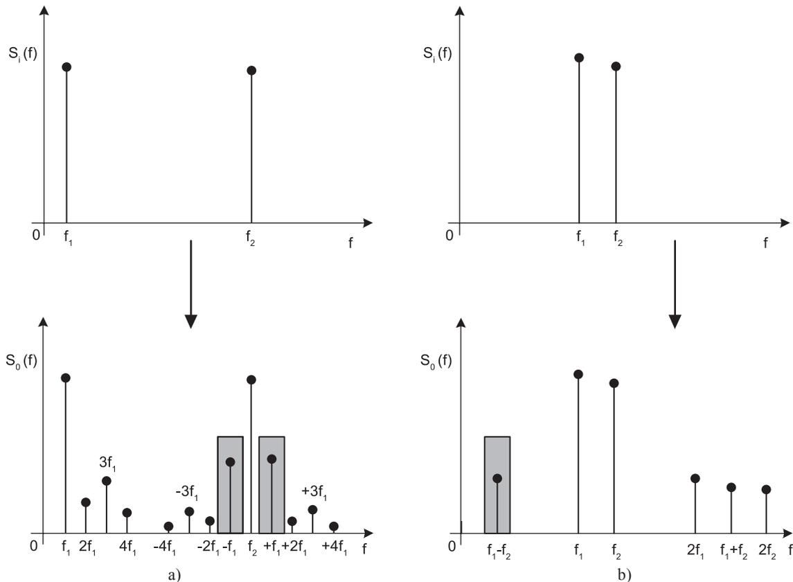
Figure 2. Creation of new harmonic components in frequency spectra at transit two harmonic signals through nonlinear environment with demonstration of selection dominant components by frequency filter. a) event of AM modulation (with large rate of  $f_2/f_1$ ), b) event of mixing (with small rate of  $f_2/f_1$ ).
