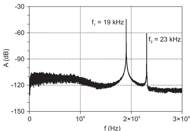
Figure 8. Response frequency spectrum of an undamaged ceiling slab, two exciting signals.
