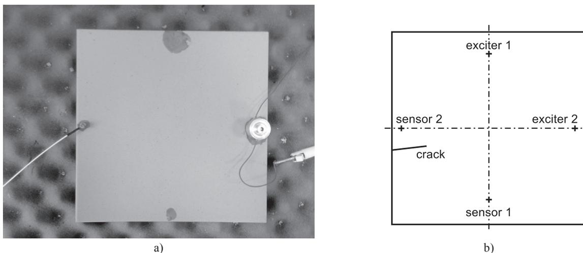
Figure 3. a) B1 specimen under test. b) Marking two positions, B2 specimen.
