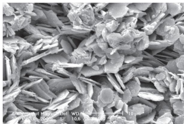
Figure 9. Platy crystals in the alumina-spinel refractory castable matrix after firing at 1500°C.
