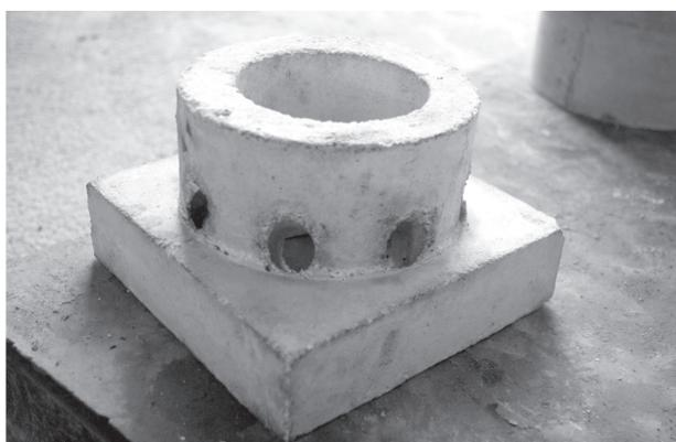
Figure 11. Pre-cast shape of alumina-spinel self-flowing refractory castable for using as burner pipe in cement kiln.
