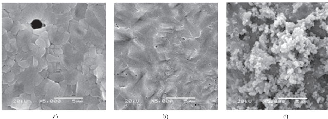
Figure 7. SEM pictures of SCPP after degradation: a) SCPP700, b) SCPP800, c) SCPP900.
