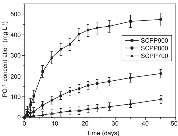
Figure 6. The phosphate ion concentration in the degradation medium for SCPP samples sintered at different temperatures.
