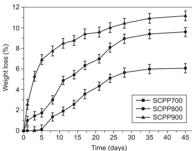
Figure 5. Weight loss of SCPP samples sintered at different temperatures.
