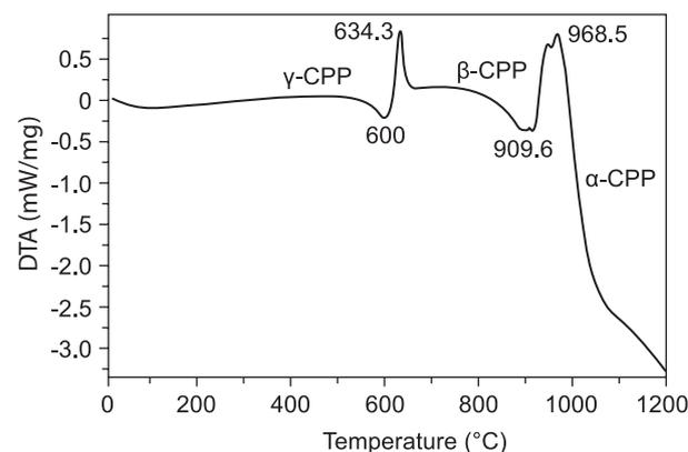
Figure 2. DTA curve of S CPP sample.
