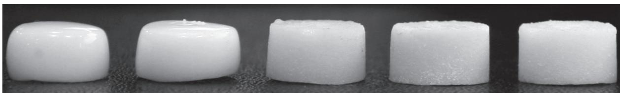
Figure 6. The profiles of compacted glasses after firing at 820°C for 10 min, from left to right, the reference, G1, G2, G3 and G4 glasses, respectively.
