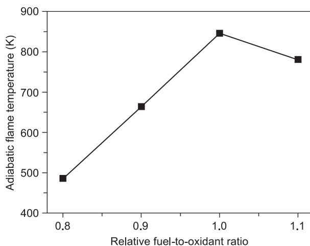
Figure 2. The theoretical adiabatic flame temperature reached during combustion as a function of the relative fuel-to-oxidant ratio.
