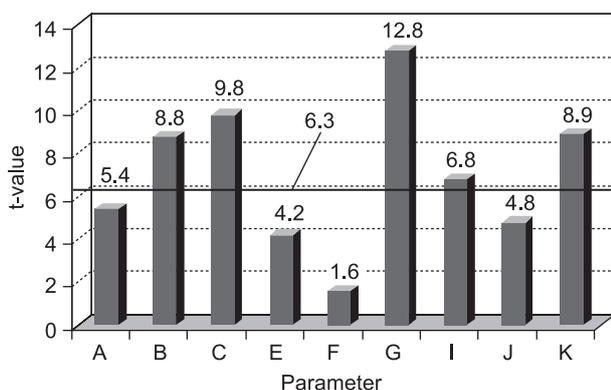
Figure 2. Standardized Pareto chart of effects on degradation of MB - estimation (SE) 0.69,  $t_{tab}(0.05, 1) = 6.3$ , 90%.
