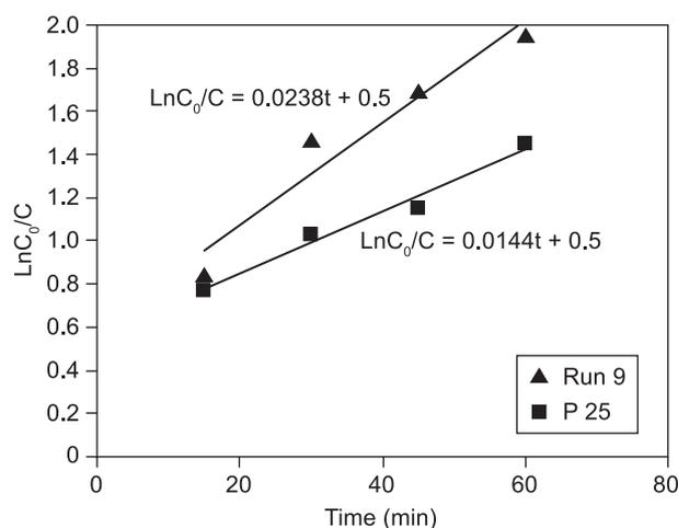
Figure 3. Dependence of the apparent rate constant ( $k, \text{min}^{-1}$ ) for sample 9 and P25.
