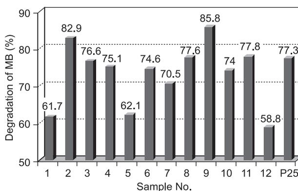
Figure 1. Degradation of MB after 60 min for prepared samples and P25.
