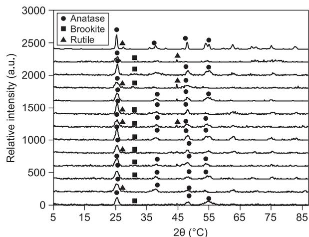
Figure 4. XRD patterns of  $\text{TiO}_2$  nanoparticles and P25.
