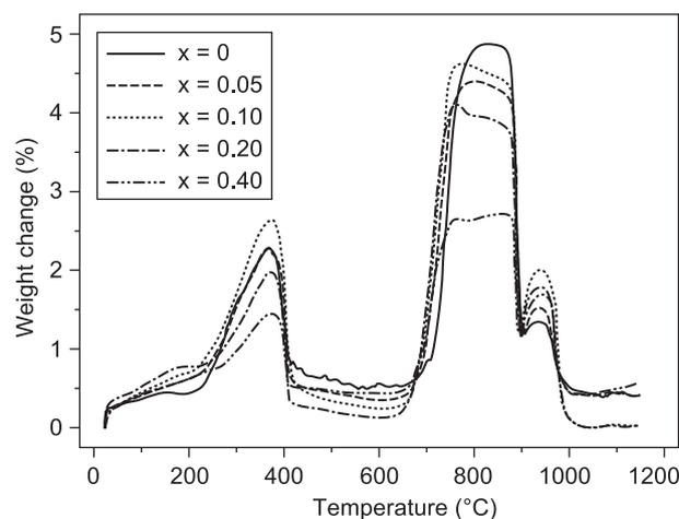
Figure 2. TG curves of Y<sub>1-x</sub>Zr<sub>x</sub>BaCo<sub>4</sub>O<sub>7</sub> in O<sub>2</sub> atmosphere.
