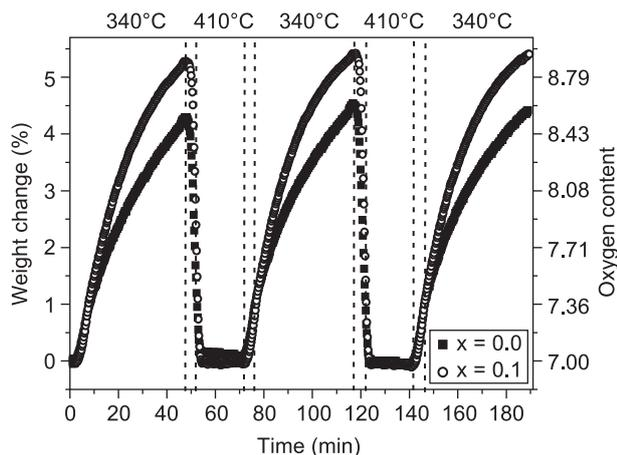
Figure 3. TG curves of  $YBaCo_4O_{7+\delta}$  and  $Y_{0.9}Zr_{0.1}BaCo_4O_{7+\delta}$  cycling between 340°C and 410°C in  $O_2$  atmosphere.
