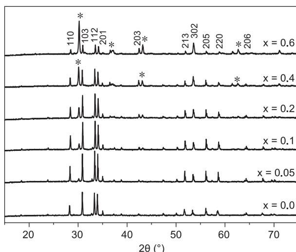
Figure 1. XRD patterns for Y<sub>1-x</sub>Zr<sub>x</sub>BaCo<sub>4</sub>O<sub>7</sub> samples.
