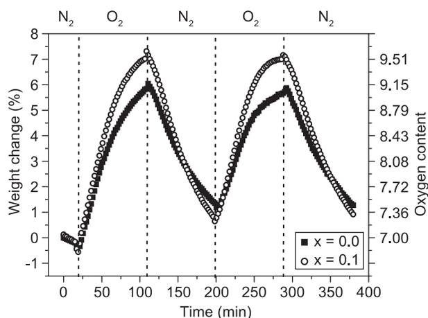
Figure 4. TG curves of  $YBaCo_4O_{7+\delta}$  and  $Y_{0.9}Zr_{0.1}BaCo_4O_{7+\delta}$  switching between  $N_2$  and  $O_2$  atmosphere at 350°C.
