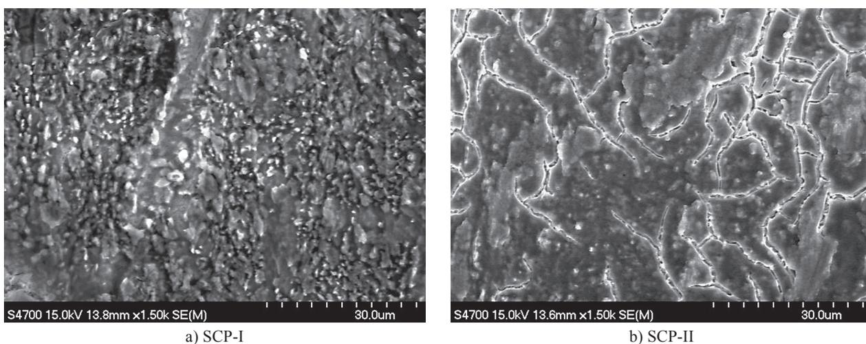
Figure 4. (SEM) Surface of coatings after firing: a) SCP-I, b) SCP-II.
