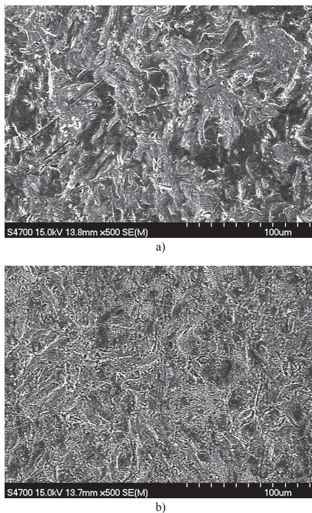
Figure 1. (SEM) Surface of titanium substrate after: a) grinding, b) leaching in HCl.
