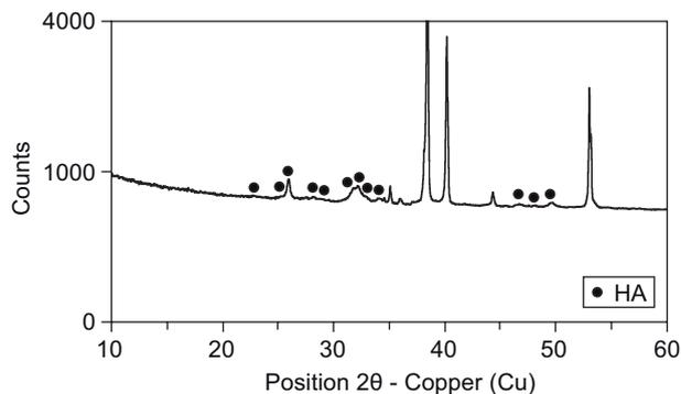
Figure 7. XRD diffraction pattern for the coating SAN after *in vitro* test.
