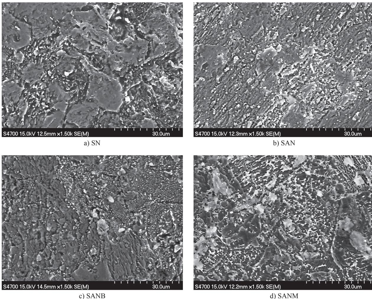
Figure 3. (SEM) Surface of coatings after treatment in NaOH: a) SN b) SAN, c) SANB, d) SANM.
