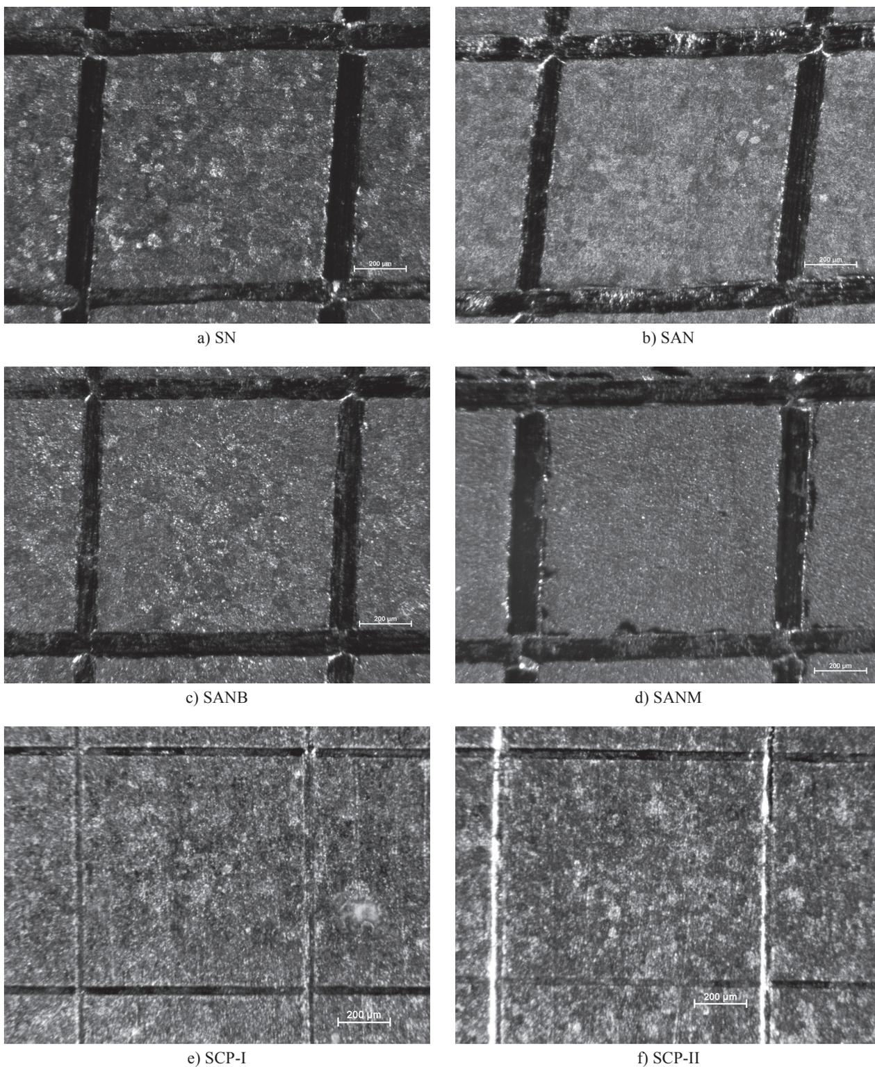
Figure 5. (OM) Coatings after tape test: a) SN, b) SAN, c) SANB, d) SANM, e) SCP-I, f) SCP-II.
