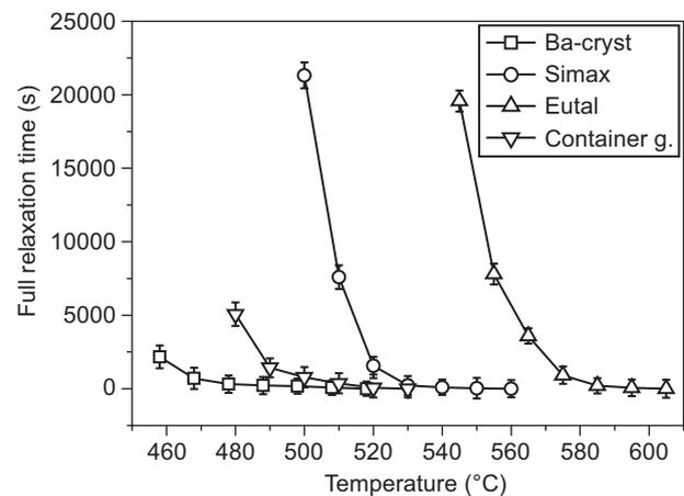
Figure 3. Full relaxation time of tension at various temperatures (heating rate 10°C/min).
