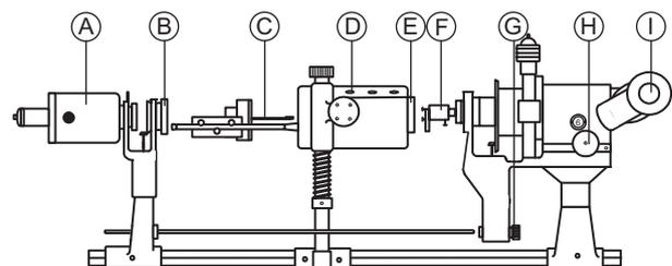
Figure 1. Measuring device (A - light source, B - polarizer, C - thermocouple, D - oven, E - monochromatic filter, F - quarter-wave plate, G - analyzer knob, H - horizontal shift, I - eyepiece).
