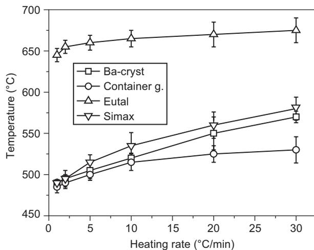
Figure 2. Temperature of full relaxation at different heating rate.
