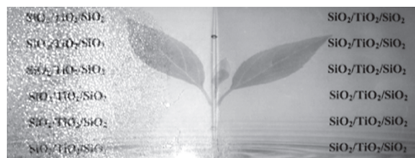
Figure 9. The photo illustrated of, antifogging glass (right) versus conventional glass (left).
