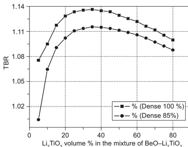
Figure A-1. TBR as a function of the Li<sub>2</sub>TiO<sub>3</sub> volume fraction for 85 % and 100 % sintered density of BeO–Li<sub>2</sub>TiO<sub>3</sub>.
