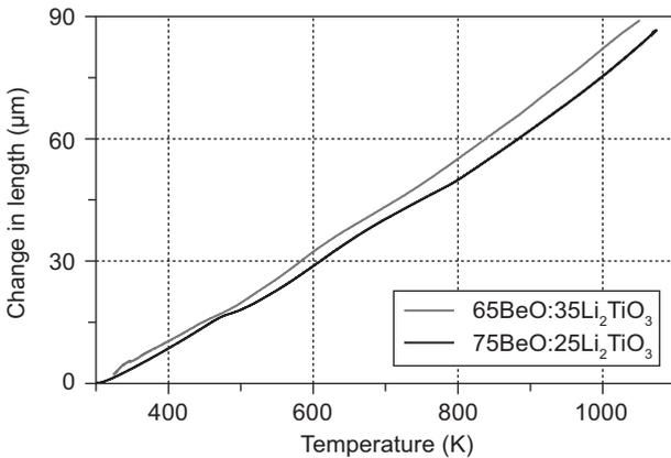
Figure 6. Change in length vs temperature plot for two compositions.
