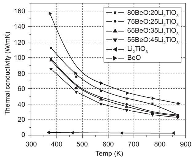
Figure 8. Thermal conductivity values for the samples.
