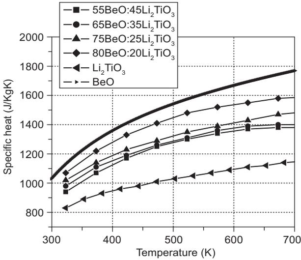
Figure 5. Specific heat variation of all the four samples with temperature.
