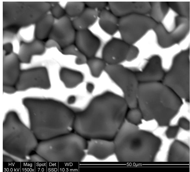
Figure 3. SEM images for a) 55 BeO:45  $\text{Li}_2\text{TiO}_3$  sample, b) 65 BeO:35  $\text{Li}_2\text{TiO}_3$ , c) 75 BeO:25  $\text{Li}_2\text{TiO}_3$ , d) 80 BeO:20  $\text{Li}_2\text{TiO}_3$ .
