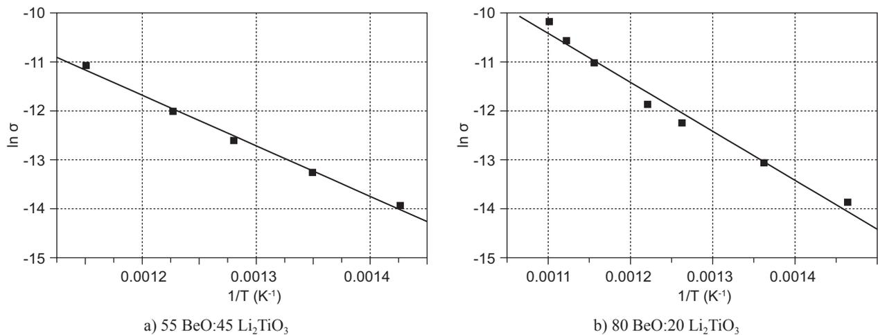
Figure 10.  $\log \sigma$  versus reciprocal temperature for a) 55 BeO:45 Li<sub>2</sub>TiO<sub>3</sub> composition, b) 80 BeO:20 Li<sub>2</sub>TiO<sub>3</sub> composition.
