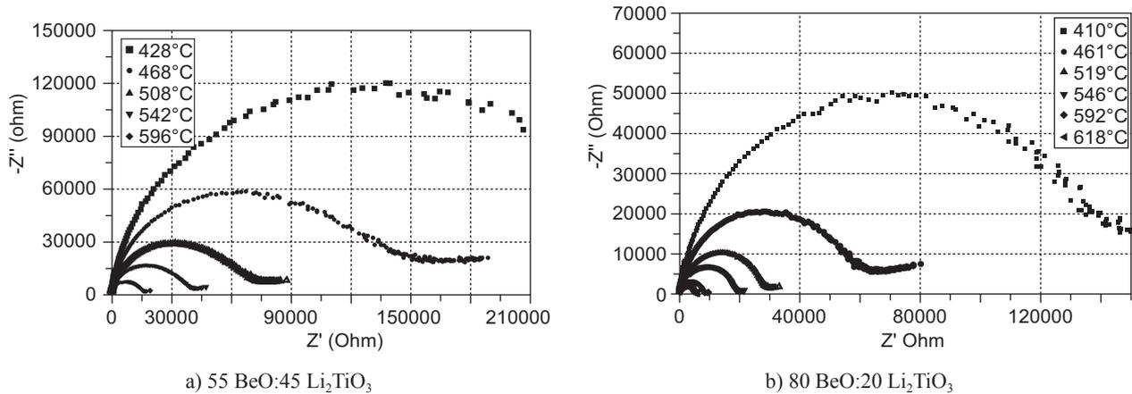
Figure 9. Nyquist plots for a) 55 BeO:45 Li<sub>2</sub>TiO<sub>3</sub> composition, b) 80 BeO:20 Li<sub>2</sub>TiO<sub>3</sub> composition.
