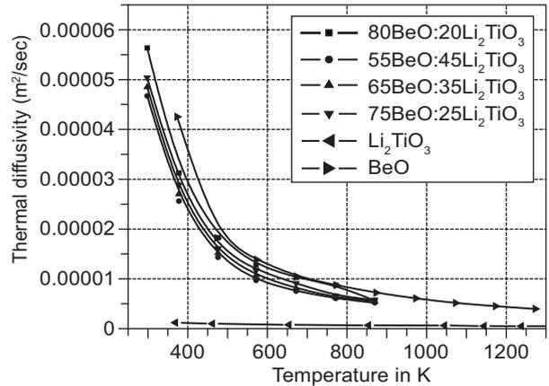
Figure 7. Thermal diffusivity values for the samples.
