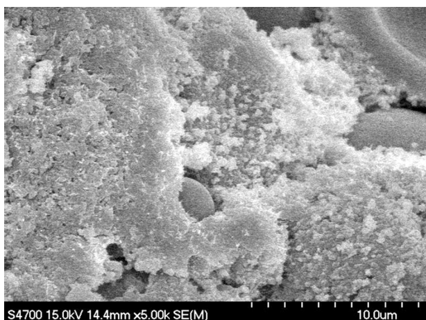
Figure 13. Geopolymer, 2 years in an environment with a relative humidity equal to 95 %, fraction surface.
