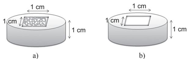
Figure 1. Schematic view of used samples for permeability test.
