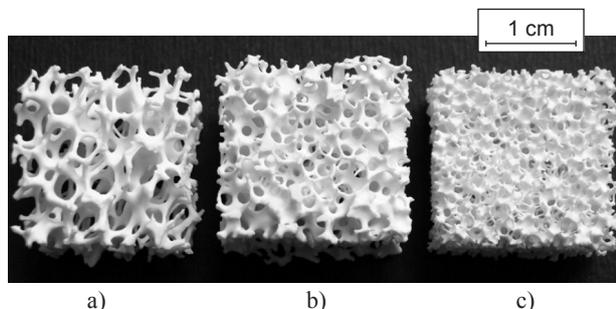
Figure 3. Morphology of alumina foams with pore density of a) 10, b) 17 and c) 27 ppi.
