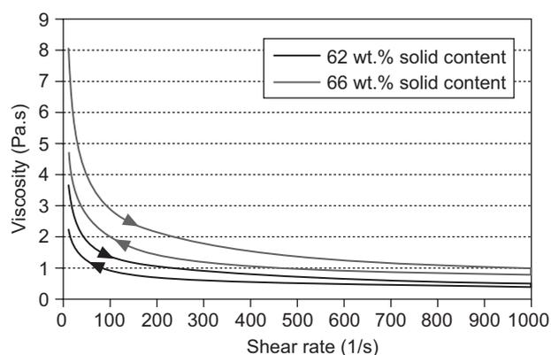
Figure 2. Viscosity curves of 62 wt. % and 66 wt. % solid content slurries.
