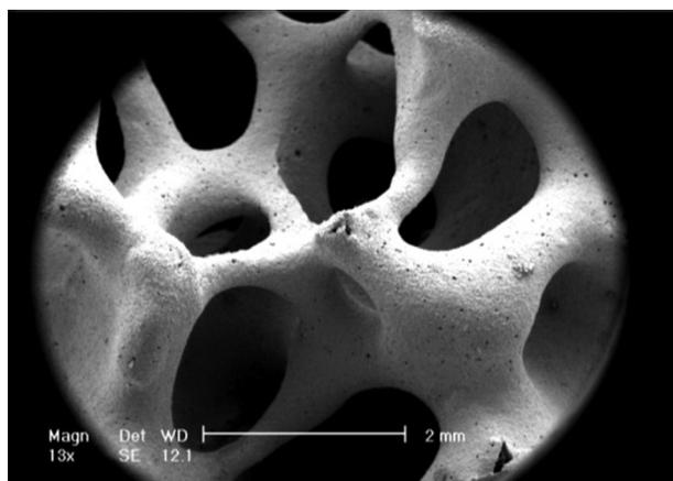
Figure 5. SEM photograph of alumina foam.
