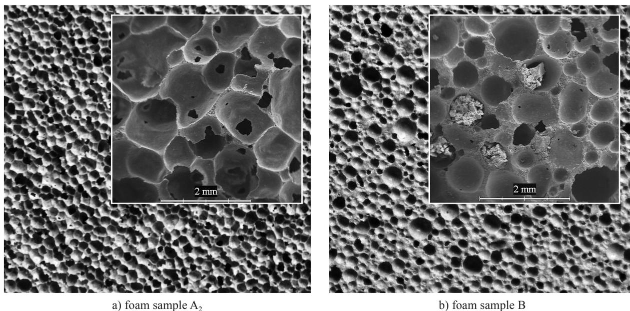
Figure 1. Microstructure of foam concrete prepared by water procedure (A2) and of foam concrete prepared by standard method (B). Middle sedimentation time (3 min) was used in this experiment.
