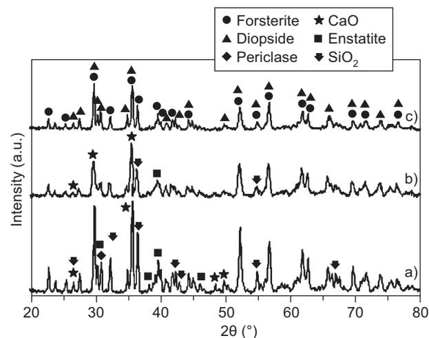
Figure 3. X-ray diffraction patterns of the prepared powder after mechanical alloying for various times and subsequent sintering at 1200°C for: a) 2 h, b) 5 h, and c) 10 h.
