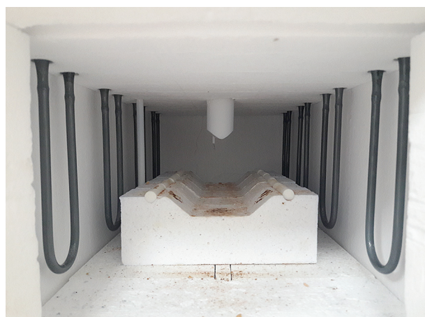
Figure 4. Detail of the interior of the device for the measurement of three-point bending.
