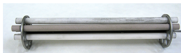
Figure 1. Placement of the samples of ceramic materials in a holder before exposure to high-temperature helium.
