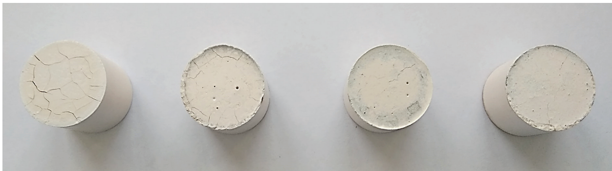
Figure 15. Photographs of the geopolymer-chitosan composites after heat treatment at 750 °C.
