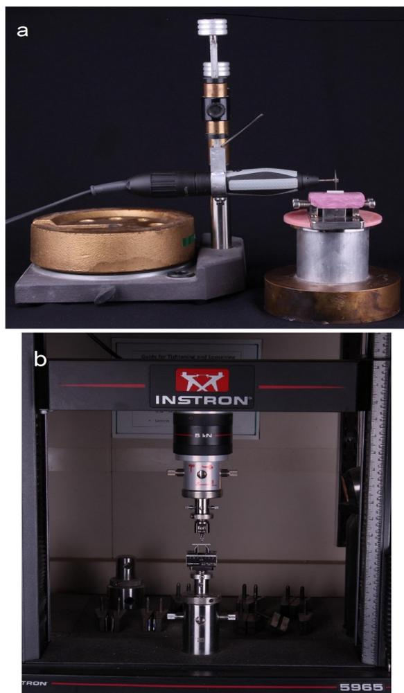
Figure 1. Preparation of the V-notch using the customised holder and diamond saw on a mounted rotary handpiece (a); Three-point bending test in a universal testing machine (b).
