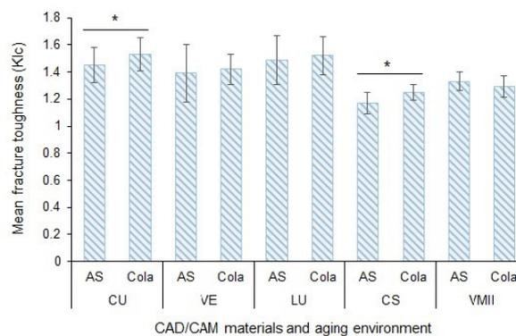
Figure 2. Mean fracture toughness of the materials aged in AS and Cola. The bars indicate the SD.
