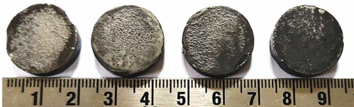
Figure 1. Images of sintered pellets of  $ZrB_2$  and  $ZrB_2$ -GNP composites. Reproduced with permission from Ref. [39].
