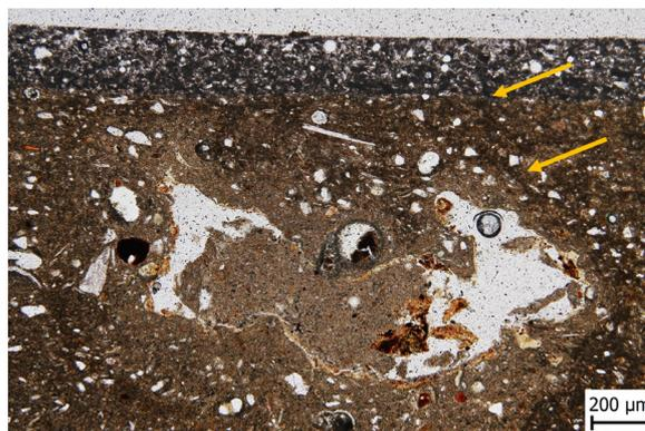
Figure 12. A detail of the thin-section of sample No. 8 with a large pore around the Ca grain continues in the form of a crack to the surface.
