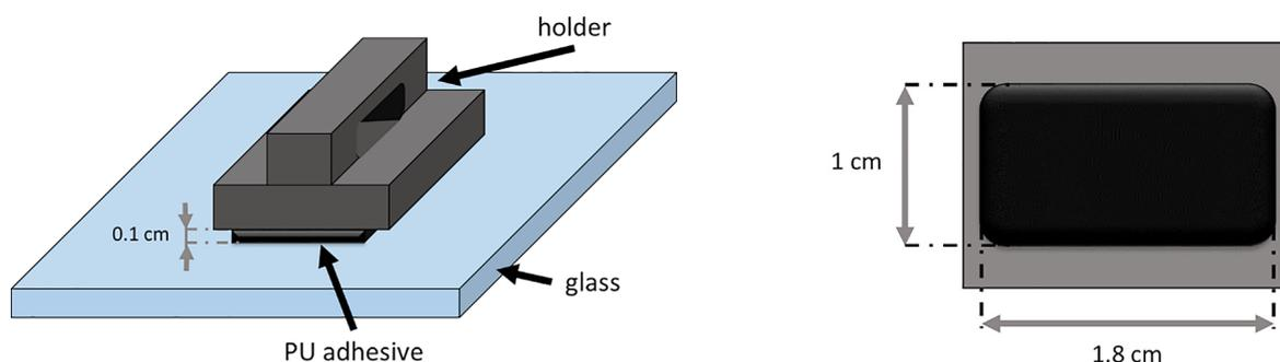
Figure 3. Illustrative drawing of the parts joined with the polyurethane glue and the final dimensions of the adhesive after gluing.
