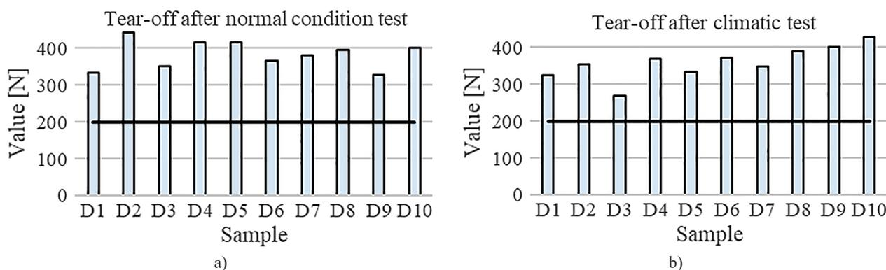
Figure 11. Graphical representation of the tear strength values performed under normal conditions and after the climatic test for the group E specimens.
