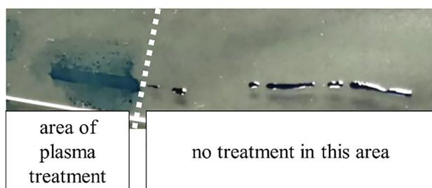
Figure 5. Photograph of a line created by a test ink with a value of  $44 \text{ mN}\cdot\text{m}^{-1}$  to determine the surface tension of the glass in the area without any pre-treatment and in the area where the point nozzle plasma was used.
