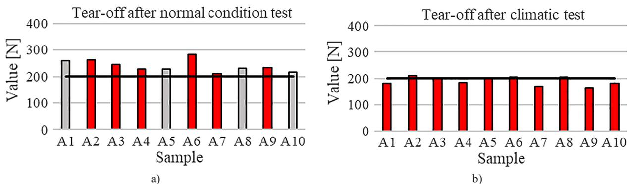
Figure 7. Graphical representation of the tear strength values performed under normal conditions and after the climatic test for the group A specimens. Samples that failed the test either because of an insufficient strength value or due to the way the connection failed are marked in red.
