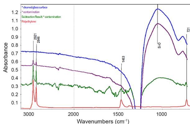
Figure 6. Typical measured reflection infrared spectra. In the area of contamination, bands of  $\text{CH}_2$  bonds (polyethylene) are visible, while these bands are not visible on the cleaned surface.
