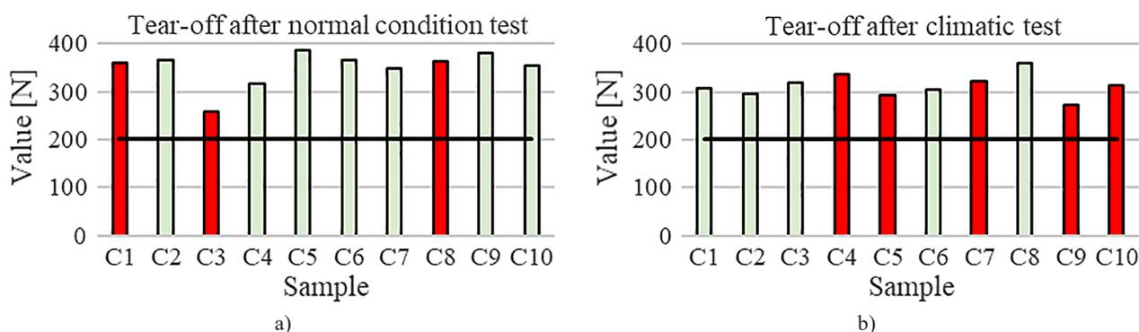
Figure 9. Graphical representation of the tear strength values performed under normal conditions and after the climatic test for the group C specimens. Samples that failed the test either because of an insufficient strength value or due to the way the connection failed are marked in red.
