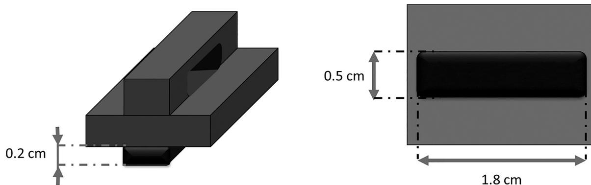
Figure 2. Dimensions of the polyurethane adhesive applied to the underside of the plastic holder.
