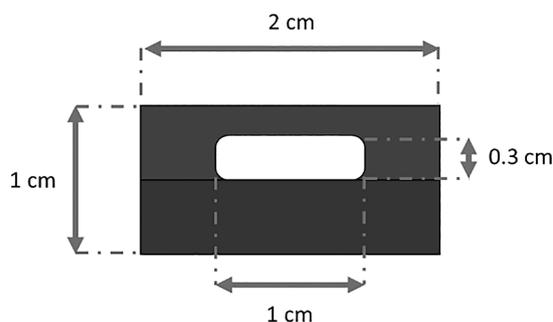
Figure 1. Dimensions of the holder made of polyamide 6 with the 30 % glass fibre content.
