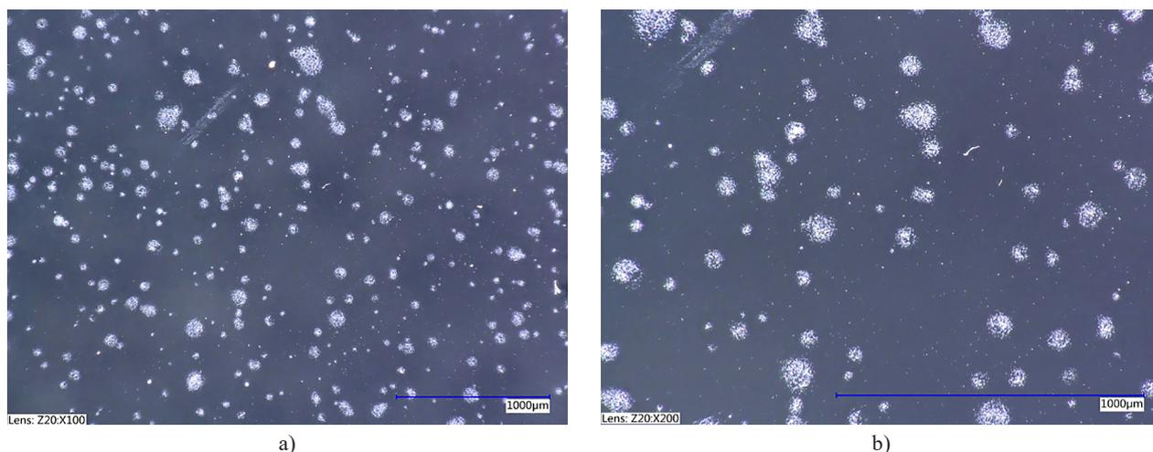
Figure 4. Photographs of the glass surface taken with an optical microscope to assess the initial cleanliness. A sample of glass sheets that had contamination on the surface.
