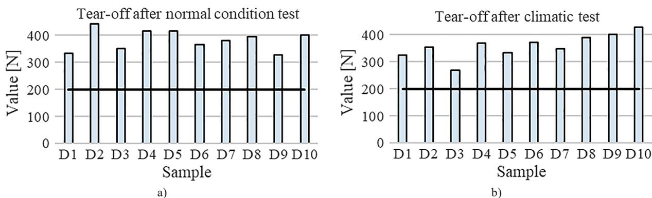
Figure 10. Graphical representation of the tear strength values performed under normal conditions and after the climatic test for the group D specimens.
