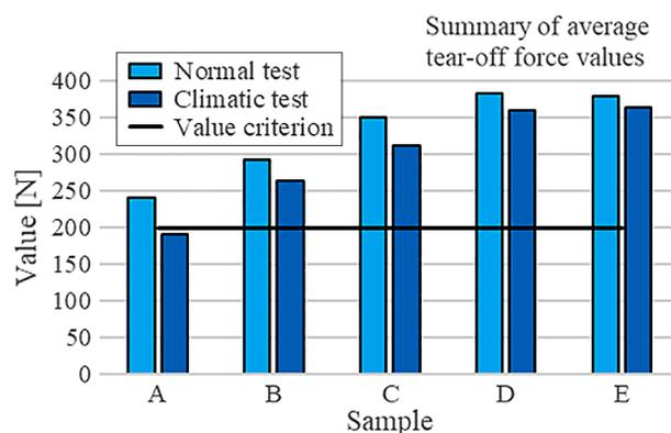
Figure 12. Summary of the average values of tear strength for the individual groups of samples marked A to E.
