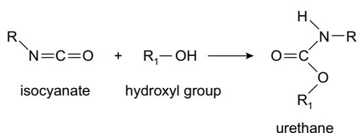
Figure 13. Schematic of a possible reaction between the functional hydroxyl group created by plasma treatment on the polyamide surface and the isocyanate group contained in the polyurethane adhesive [22].
