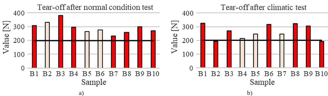
Figure 8. Graphical representation of the tear strength values performed under normal conditions and after the climatic test for the group B specimens. Samples that failed the test either because of an insufficient strength value or due to the way the connection failed are marked in red.
