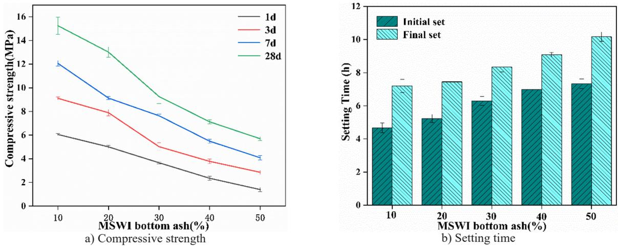
Figure 5. The effect of adding MSWI BA to fly ash.
