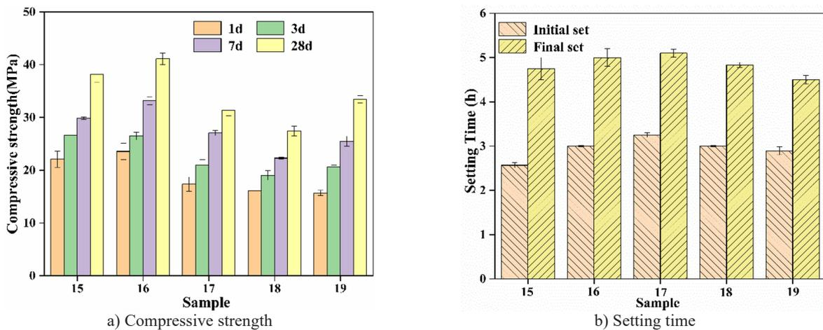
Figure 8. Research on the performance of the cement and mineral powder mixed in the MSWI BA.
