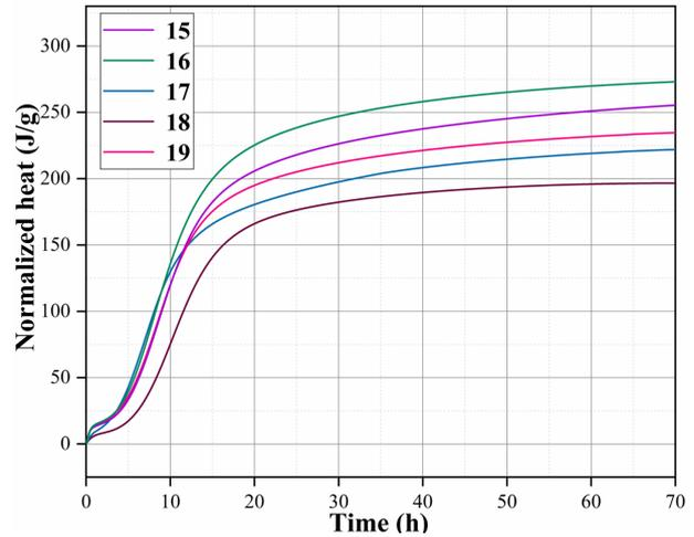
Figure 12. Hydration heat release curve.
