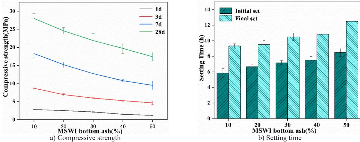
Figure 7. The effect of adding MSWI BA to cement.
