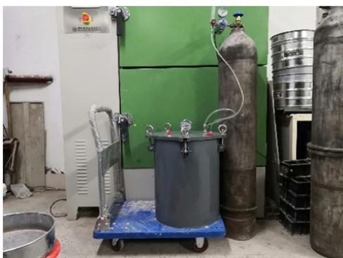
Figure 1. The carbonation device.
