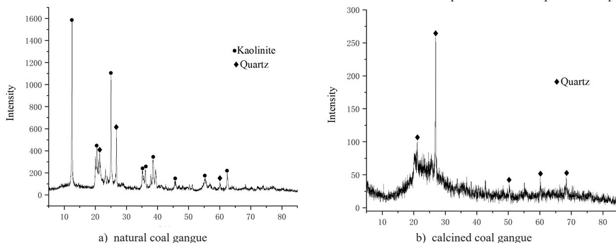
Figure 3. XRD patterns of the natural coal gangue and calcined coal gangue [26].
