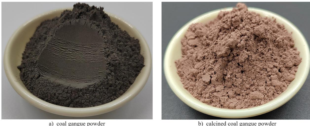
Figure 1. Coal gangue powder before and after calcination.
