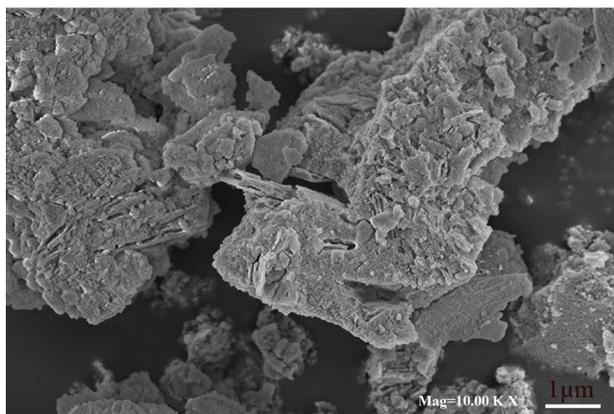
a) low magnification SEM for the lowest strength geopolymer
