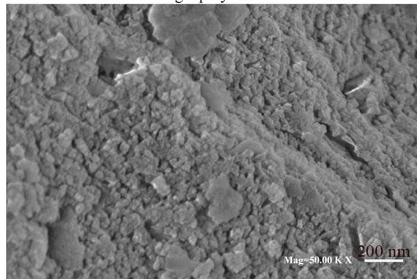
d) High magnification SEM for the highest strength geopolymer
