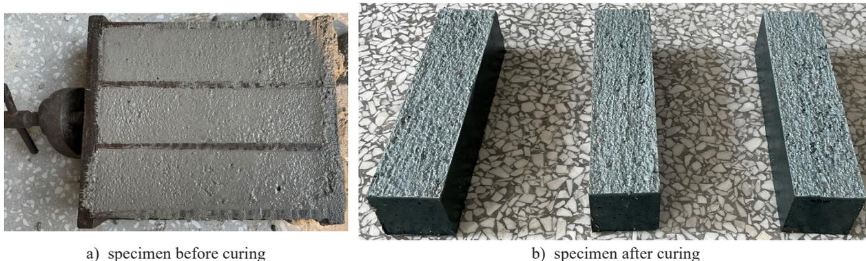
Figure 2. Coal gangue-based geopolymer before and after curing.
