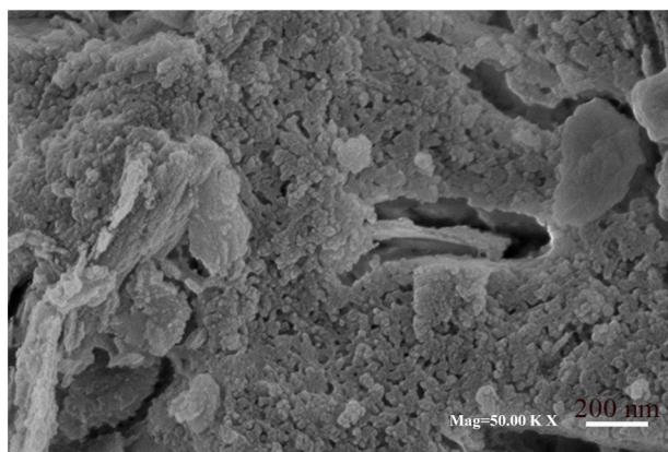
b) high magnification SEM for the lowest strength geopolymer
