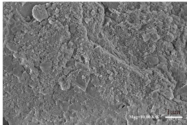
c) Low magnification SEM for the highest strength geopolymer
