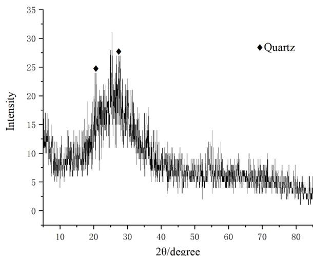
Figure 4. XRD pattern of the coal gangue-based geopolymer at 28 days of curing [27].
