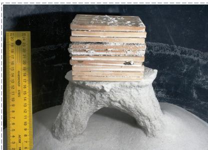
Fig. 4: Result of experiments with Strelce sandstone - a perfect experimental gate, formed by repeated flooding of a loaded block with a rectangular opening.
