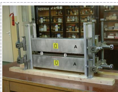
Fig. 5: A-tubes with sets of magnets, B - Air gap with strong magnetic field, C - devices to control the width of the air gaps, D - bolts to adjust the magnet sets
