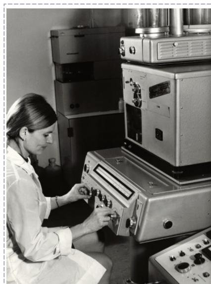
Measuring the parameters of the thermal decomposition of coal
