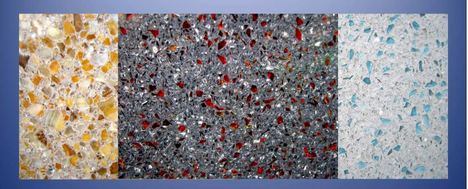
The Geopolymer composite with the colored glass and mirror shards in pigmented matrix.
