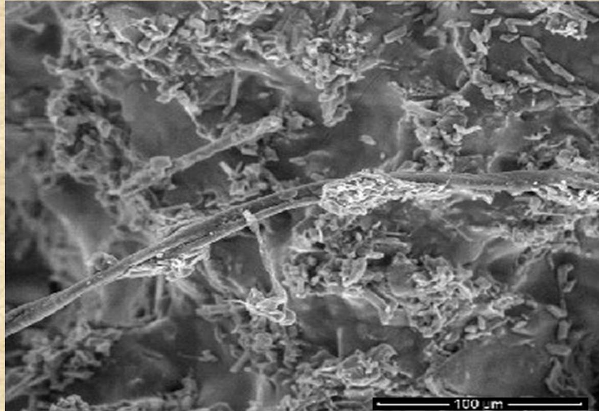
Across the picture we could observe twisted fiber with small particle glued on it.
