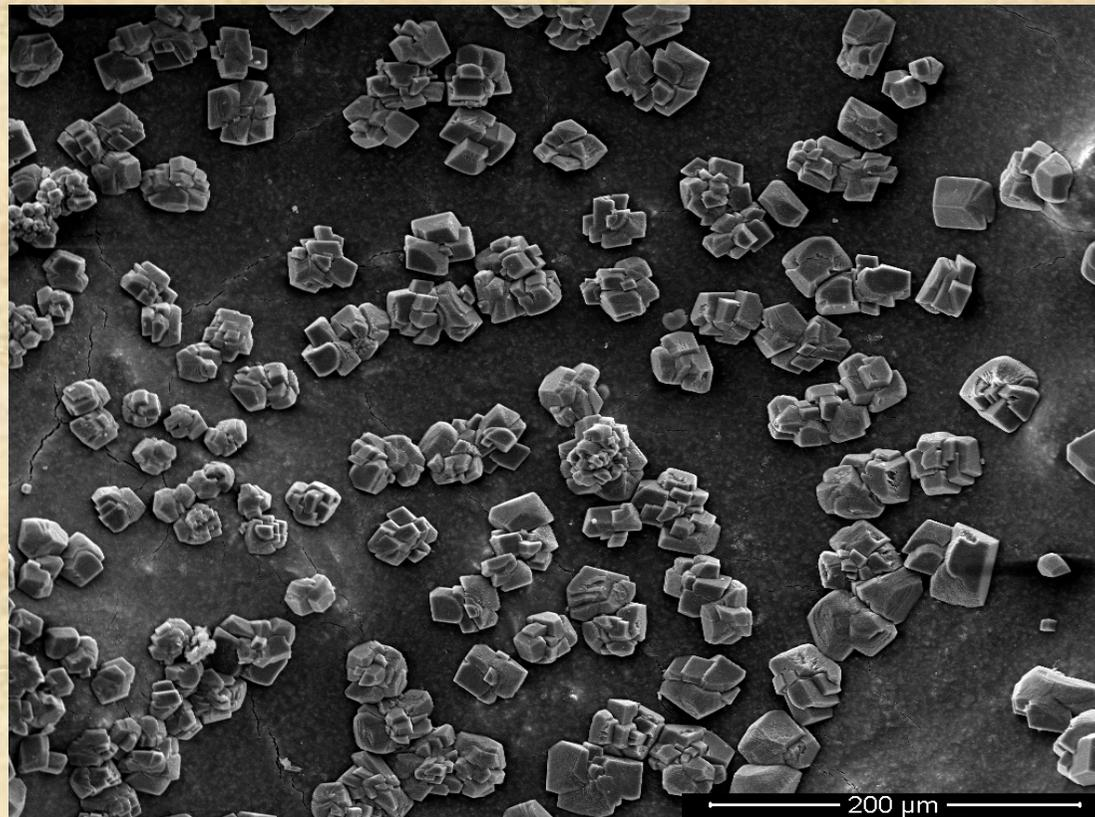
Crystals of gehlenite identified also by XRD analysis (bottom of convex part of a big pore)
