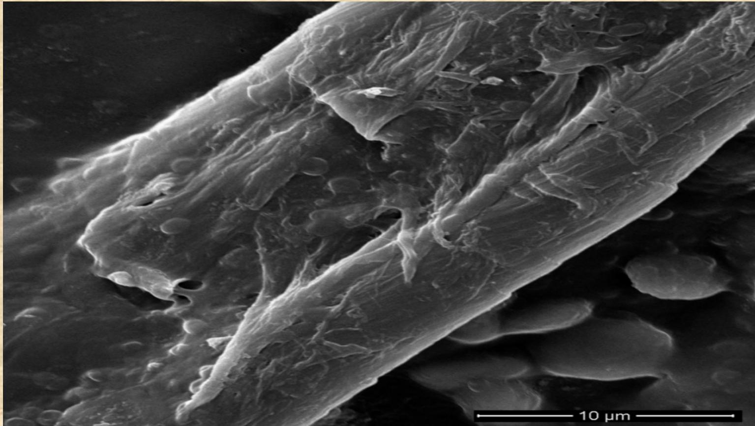
The borders are rounded and stronger than central part of the fiber and probably these differences produce twisting effect of the fibers.
