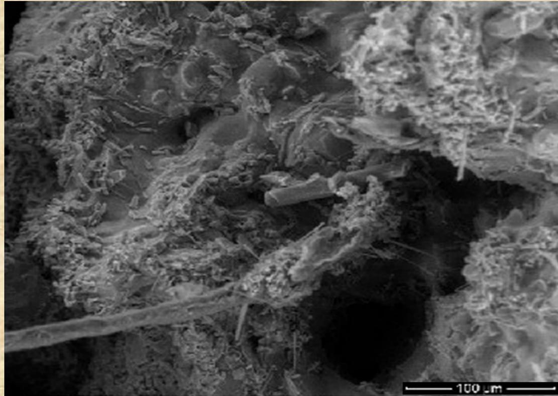
The SEM picture shows one of the nascent point of one long and one broken fiber, some small and thinner fibers are also detected (right part of the picture).
