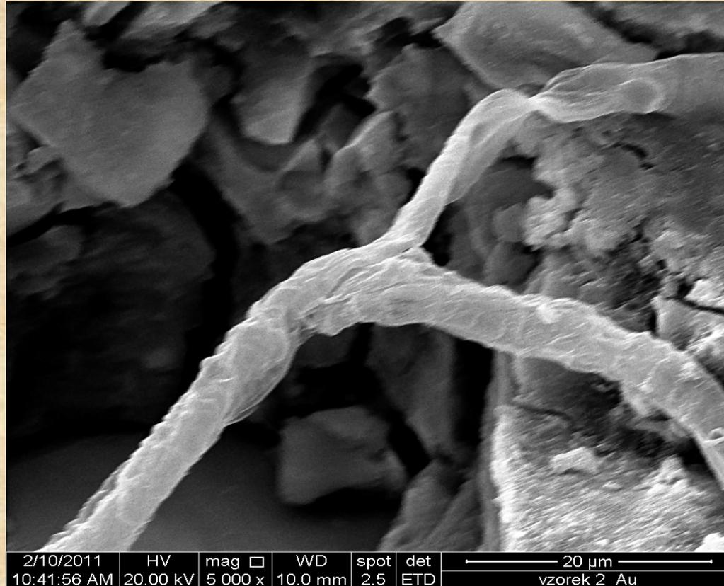
The fiber is crossing the pore - visible highly heterogeneous structure of the surroundings.
