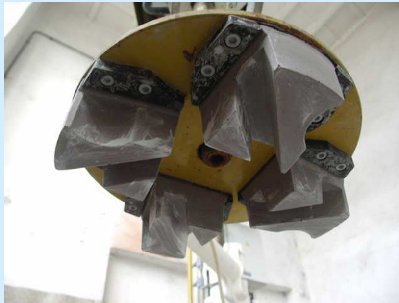
Semi-industrial grinding: Grinding stones fixed in holder
