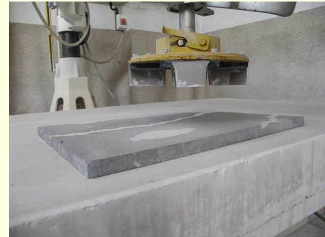
Machine prepared for grinding
