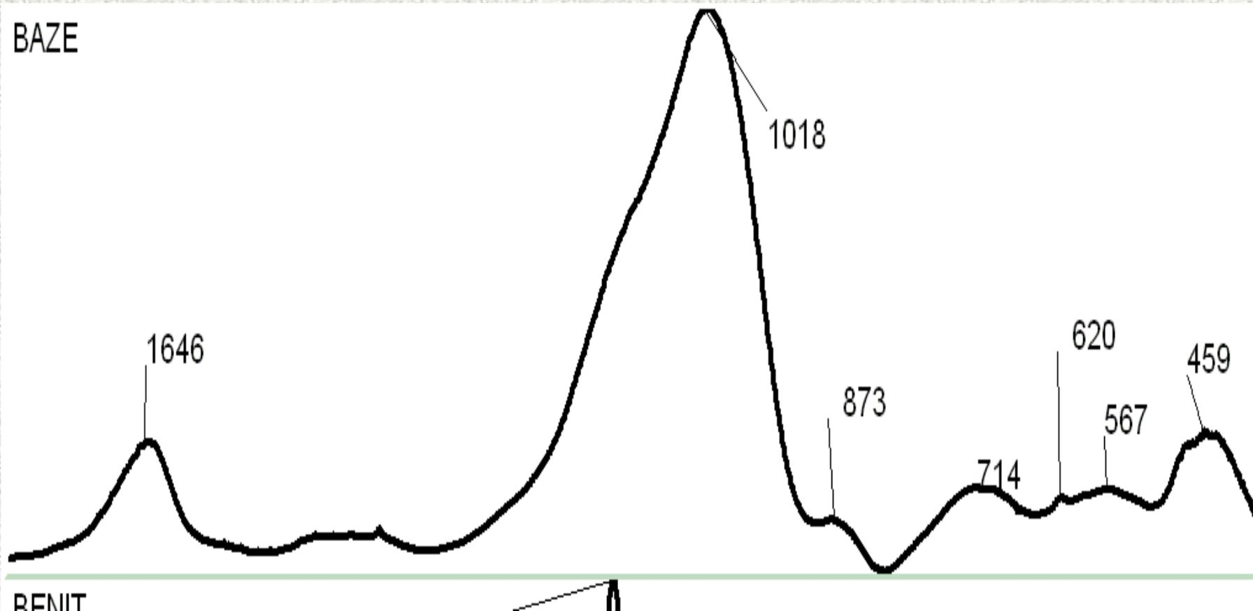
Vibrations at 1018 cm<sup>-1</sup> is a proof of geopolymer Si-O, Al-O bonding
