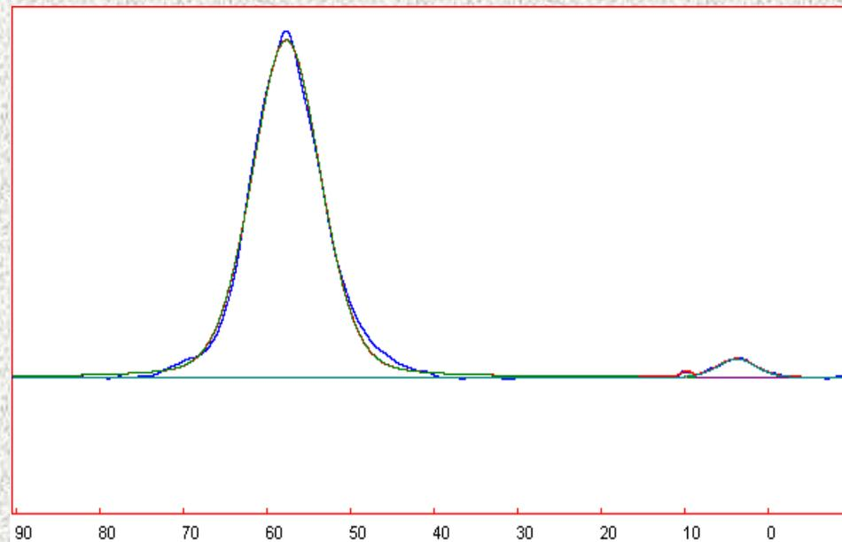
Geopolymer prepared from activated Czech kaolin Sedlec Ia – all alumina ions are tetra coordinated in respect to oxygen (= 58 ppm ).
