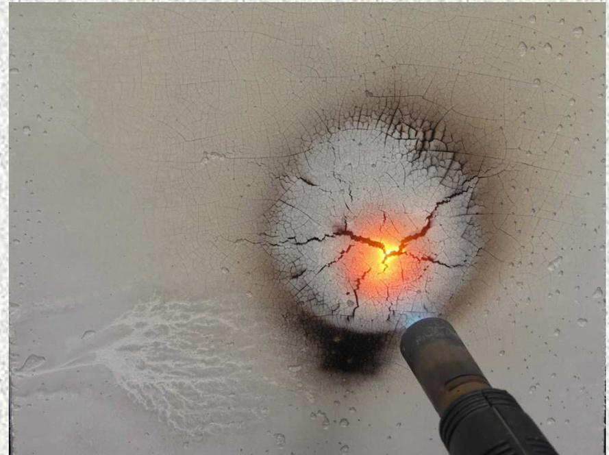
The geopolymer composite made from alternated layers of geopolymer and cotton fabrics. Hot side + 900 °C , thickness of the plate 12 mm and resistance measured expressed in minutes when cold side temperature reaches 140°C. Time was 8 minutes 57 seconds. Distance of the burner 5 cm (pict.2) and 15 cm (pic.1) when the resistance grows up to 38 minutes.
