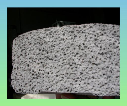
Resistance to 1200°C without shrinkage or cracks
