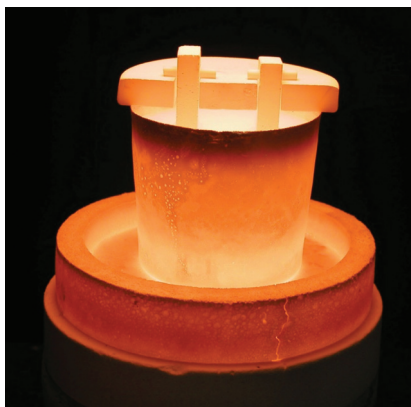
Crucible with refractory material corroded by glass melt
