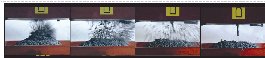
Successive phases in the attraction of steel screws from beneath an 80-90 mm layer of crushed stone from a distance ca 200 mm towards the surface of the suspended magnetic circuit.
