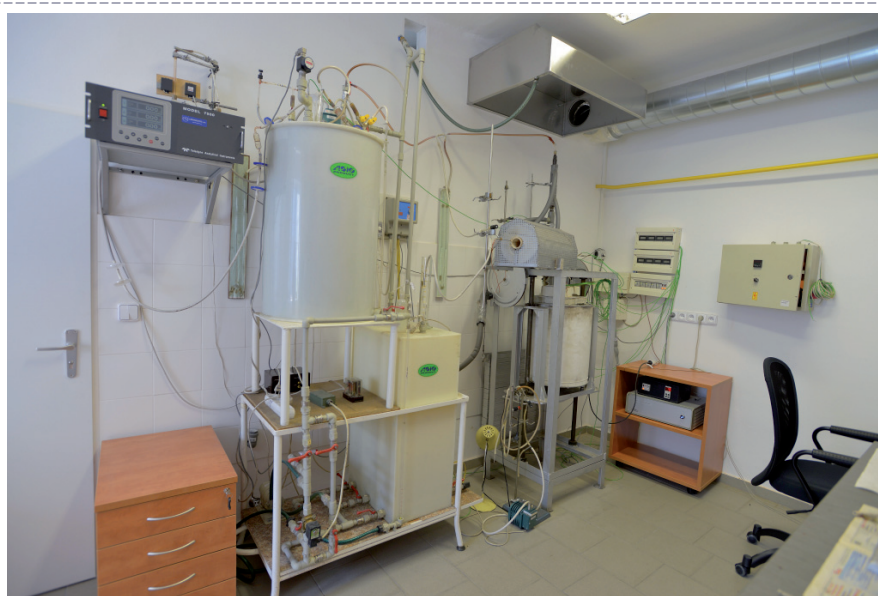
Heat-treatment furnace with fixed bed and cracking module
