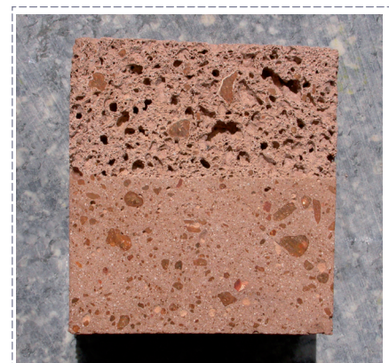
A solid product from a foamed and non-foamed geopolymer containing a high amount of aluminum-production waste
