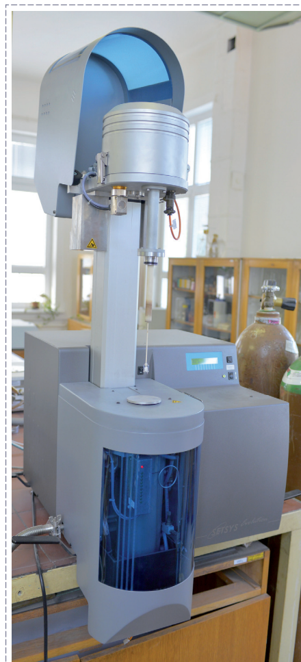
Thermal analyser SETARAM Setsys Evolution No. 18 working in both inert and oxidizing atmospheres
