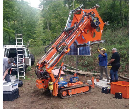
Installation of a DMS multiparametric inclinometer by CSG at the Čeranišřt landslide site (CZ)
