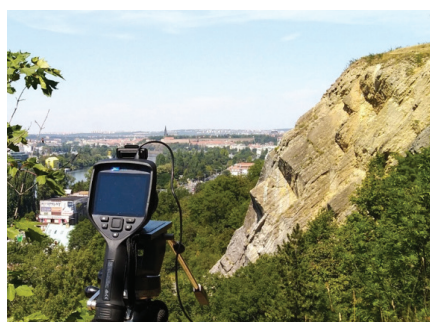
Time-lapse monitoring of the rock surface temperature at Branická skála using an IR camera (Prague, CZ)
