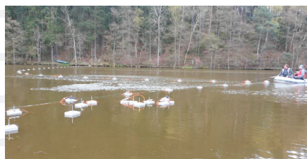
ERT measurement of landslide-dammed lake sedimentary infill across Mladotice lake (CZ)
