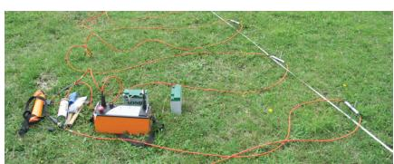
ERT measurements using the ARES resistivity system. Searching for the Sudetic Marginal Fault - its location and trace at Bílá Voda site
