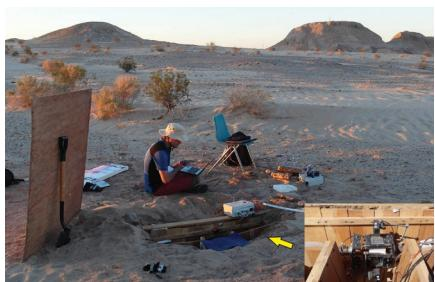
Displacement monitoring on the Superstition Hills Fault, California, using a TM71 mechanical dilatometer with automated data recording
