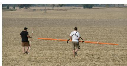
Conductivity measurements using the CMD Explorer serve as a powerful tool for determining the areal extent of sedimentary features (e.g. alluvial fans, colluvial deposits, etc.)
