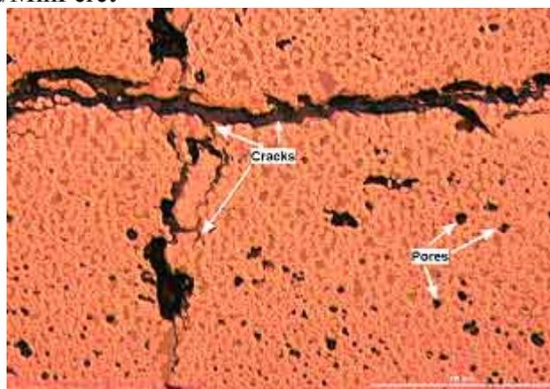
Fig 5. Porous system of 2D C-C composite
