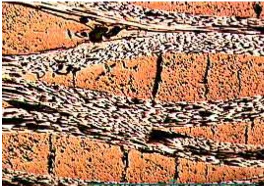
Fig 1. 2D C-C composite cross-section.
