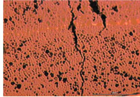
Fig 4. 2D C-C composite cross-sections, magnification 200x
