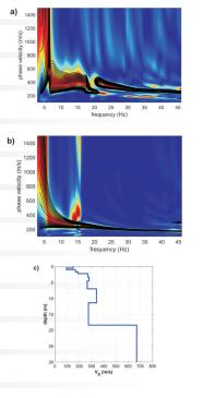
Velocity model retrieved from measurement and analysis of phase velocity
