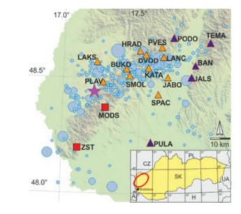
The MKnet seismic network monitors seismic activity in the Malé Karpaty region. The blue circles symbolize earthquakes. The historical 1906 earthquake of magnitude 5.7 is shown by the big purple star. The stations JALS, BAN, PODO, PULA and TEMA are provided by IRSM CAS.
