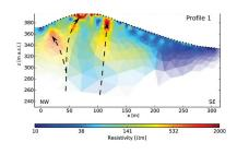
Two-dimensional inverted resistivity (electrical resistivity tomography) image of the Zebín Volcano along profile 1. The lowresistivity zones (up to approximately 100  $\Omega$ m, blue and bluish colours) represent clayrich sediments, whereas the high resistivity areas (approximately 300  $\Omega$ m and more, red colours) represent coherent basic dikes. The possible magma feeder conduits/dikes are indicated by dashed arrows.
