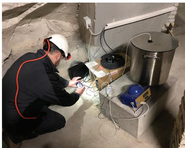
Installation of Rotaphone station near Litoměřice
