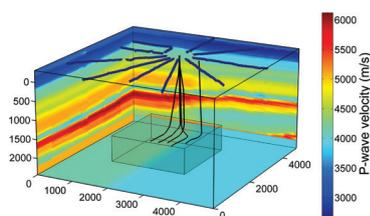
3D P-wave velocity model, wells and surface star-like monitoring array acquiring microseismic data during hydraulic fracturing in shale
