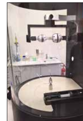
This 4SPIN device by Contipro a.s. is used for electrospinning polymer solutions, especially with polymers of natural origin such as collagen, or for coating implants; the image shows sockets for a hip prosthesis. Photos by Vlasta Mádlová and Tomáš Suchý.
