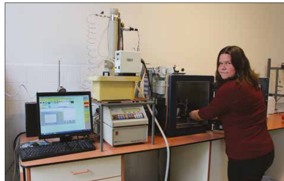
Daniela Římnáčová working with a high-pressure sorption device. Photo by Vlasta Mádlová.
