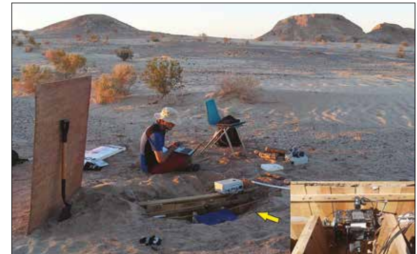
Check upon the TM-71 dilatometer that automatically registers displacement on the Superstition Hills fault at the Imler monitoring station in South California. Undated. Photo by Petra Štěpančíková. IRSM.
