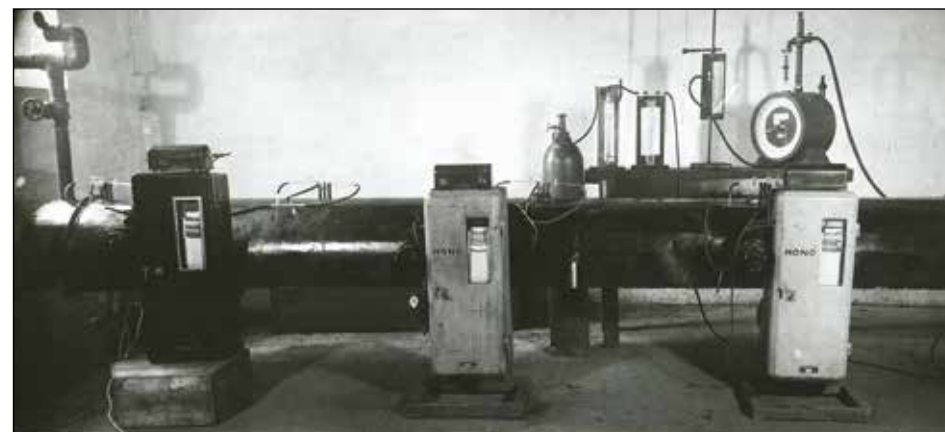
Studies on the diffusion of methane and CO 2 were carried out in vertical cylinders or in a horizontal laboratory tunnel. Department of Gas. Photograph from the Institute's 1952 annual report. NA Archives, Ministry for Fuels and the Power Industry collection, box 110, inv. no. 84.
