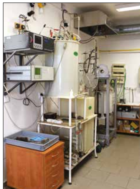
Olga Bičáková preparing a device for the thermal processing of organic waste materials. Furnace with a stationary bed and second stage, 2018. Photo by Vlasta Mádlová.
