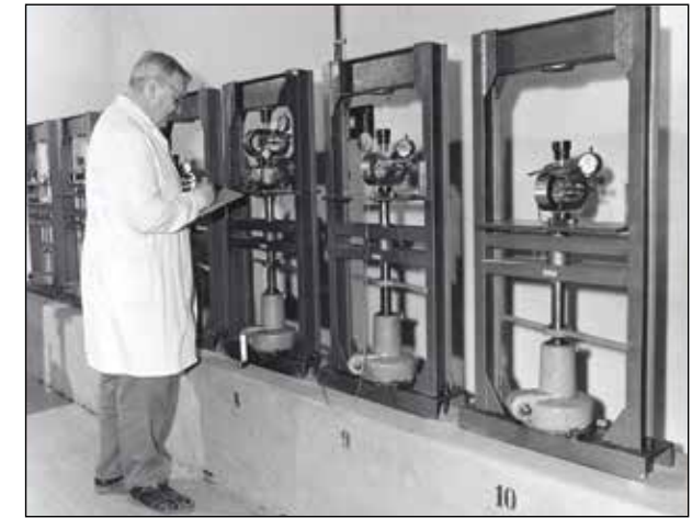
Long-term rheological tests of rocks under simple compression on spring power presses, Jaromír Houska, undated. Photo by Renáta Louvarová (Záběhlická). IRSM, collection of photographs.
