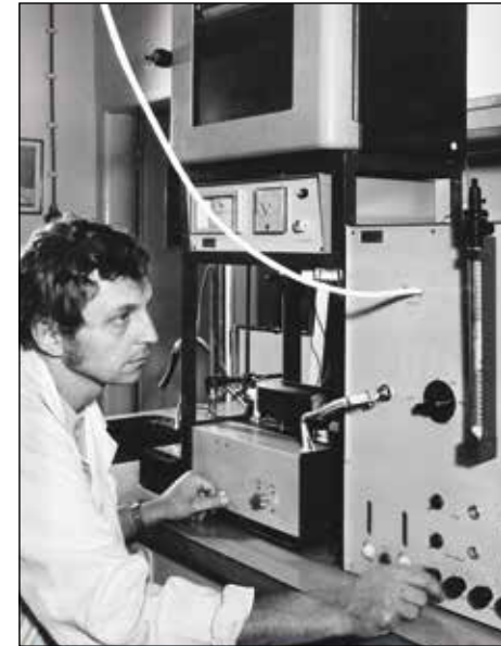
Measurement of gaseous pollutants on a chromatograph, Václav Štochl, undated. Photo by Renáta Louvarová (Záběhlická). IRSM, collection of photographs.
