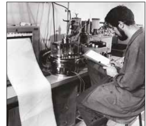
Petr Glogar measuring the thermal conductivity of rock samples from the Příbram uranium ore deposit. The measurement of this variable was fundamental for the thermal exchange (heating) of the mine atmosphere in the deep horizon where the temperature exceeded 35°C and an expensive cooling system for the atmosphere was therefore required. P. Glogar designed and made this device.
