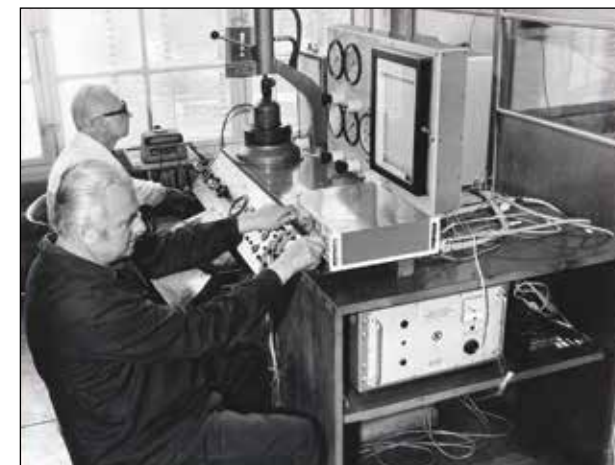
ČSAV Mining Institute employees Žampach and Polák – rock tests in a triaxial device under multiaxial stress, tensometric measurement of deformable characteristics, undated. Photo by Renáta Louvarová (Záběhlická). IRSM, collection of photographs.
