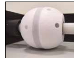
This 4SPIN device by Contipro a.s. is used for electrospinning polymer solutions, especially with polymers of natural origin such as collagen, or for coating implants; the image shows sockets for a hip prosthesis. Photos by Vlasta Mádlová and Tomáš Suchý.
