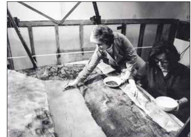
Bottom stability measurement of the Jiří Mine on a model, Sokolov region, Eva Jeníková, Hana Košťálová. Photo by unknown author. IRSM, collection of photographs.
