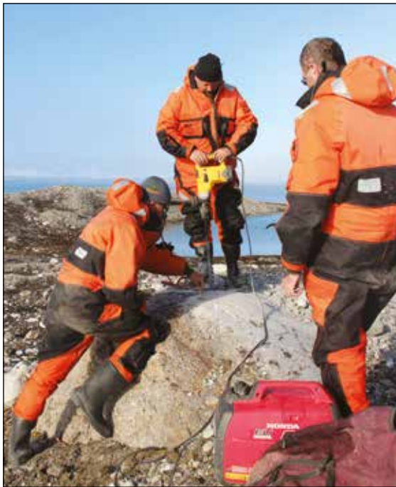
Josef Stemberk, Filip Hartvich and Jan Blahůt installing a GNSS point to measure geodynamic movements at Hornsund fjord, undated. Photo by M. Hladká. IRSM.
