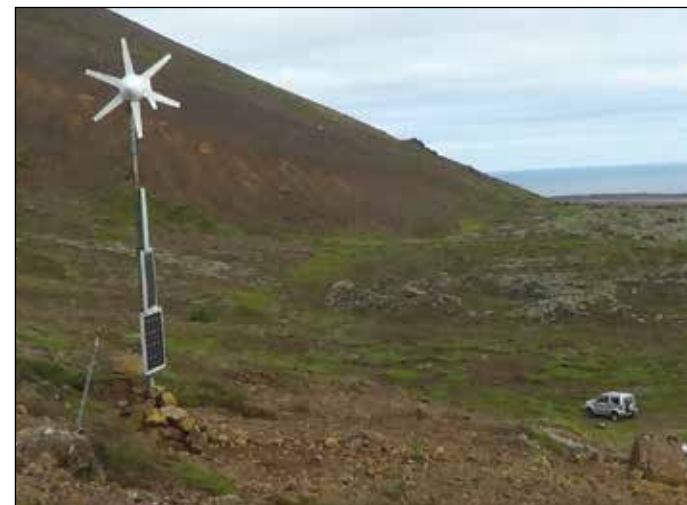
Seismic station in southwest Iceland, part of the REYKJANET network operated by the Institute of Geophysics and the Department of Seismotectonics of the IRSM, undated. Photo by unknown author. IRSM.
