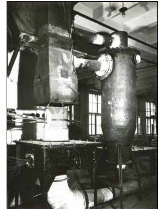
Thermal and technical research group. Experimental laboratory equipment for research into the combustion process in a fuel layer on a grate, developed in 1951. Photograph from the Institute's 1952 annual report. NA Archives, Ministry for Fuels and the Power Industry collection, box 110, inv. no. 84.
