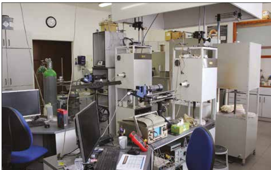
Laboratory ovens for the high-temperature monitoring of processes in molten glass, 2018. Photo by Vlasta Mádllová.
