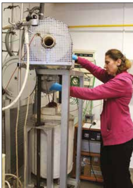
Olga Bičáková preparing a device for the thermal processing of organic waste materials. Furnace with a stationary bed and second stage, 2018. Photo by Vlasta Mádlová.
