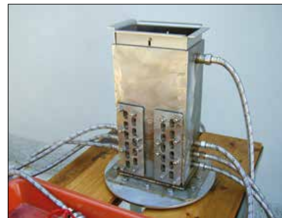
Device for setting up magnets into blocks with high magnetic field values, patented in the USA, undated. Photo by unknown author. IRSM.
