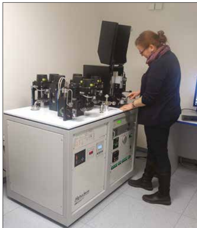
The Alphachron TM mass spectrometer designed for helium thermochronology, which uses automated extraction of radiogenic helium and can measure its contents in samples of minerals. Undated. Photo by Petra Štěpánčíková. IRSM.
