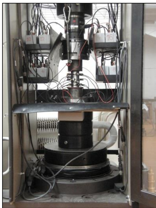
Fig: Loading a cylindrical rock sample using the uniaxial compression strength measurement method while simultaneously detecting failure using acoustic emission.
