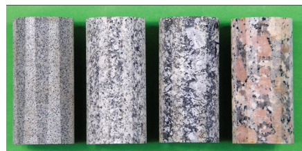
Four specimens before testing, from left to right: westerly granite, mrakotin granite, Brno syenite, and liberec granite
