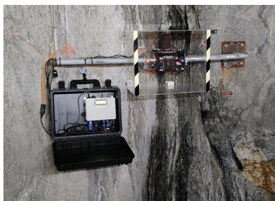
The 3D crack gauge TM72 monitors deformation in the Grimsel Test Site, 450 metres beneath the surface of the granite Aar Massif. Since 2012, the monitoring has been performed in collaboration with NAGRA (CH) and RAWRA (CZ).
