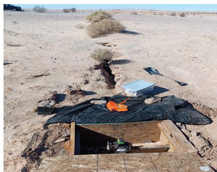
Monitoring of displacements along the Superstition Hills Fault (see the fissure) carried out by extensometer TM71 with automated .data recording.
