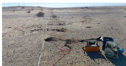
Electric resistivity measurements using ARES resistivity system. Searching for the Superstition Hills fault, southern California.
