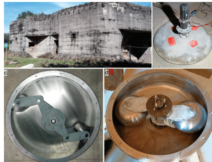
Prototype of a seismic beacon installed in an old military bunker
