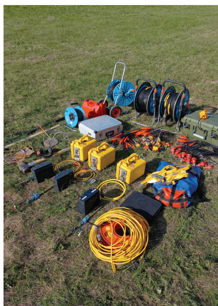
Equipment for the acquisition of surface wave data for site characterisation (Geode).
