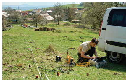
Field work – acquisition of surface wave data for site characterisation.
