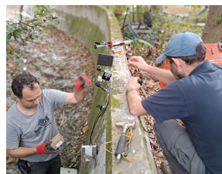
Installation of a novel contactless 3D positioning system on the Chihshang plate-boundary fault in Eastern Taiwan (photo by J. J. Dong).
