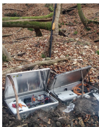
Controlling unit and the measuring device of the permanent electric resistivity profiling are hidden underground in water-proof boxes.
