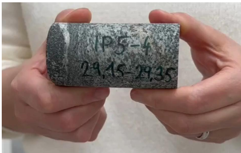
Illustrative photograph: Sample used to test the bedrock of the Dukovany II Nuclear Power Plant.
